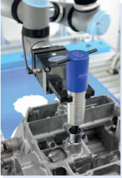
Automatic Measuring Cell: autonomous, robot based measuring with a plug gauge
