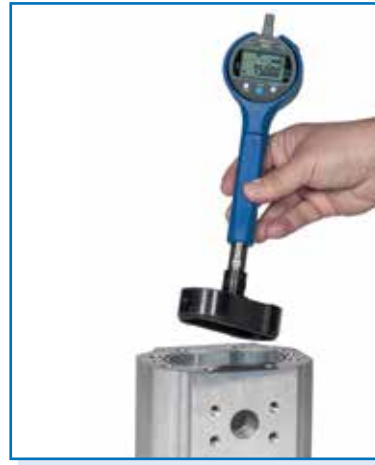
2-point internal measuring instrument in action
