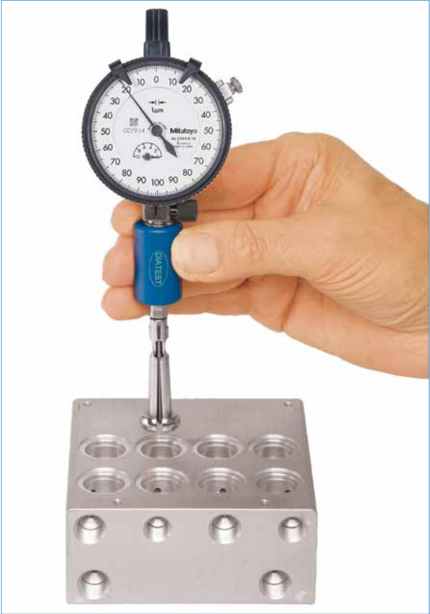
2-Point Inside measuring instrument in action
