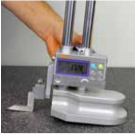
Excessive downwards force lifting the base from the plate
