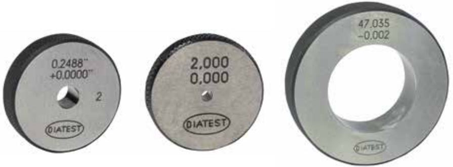
Examples for DIN 2250-C setting rings (metric and inch)
